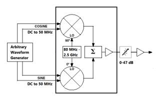
At the heart of the VSG25A is a quadrature modulator driven by an arbitrary waveform generator consisting of 2, 12-bit DAC channels, a direct digital synthesizer (DDS), and pattern memory. The waveforms represent the I and Q channels of the complex signal to be produced.
