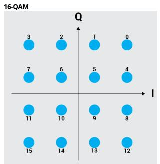
*Note: Positive I-axis is to the right, positive Q-axis is to the top.*
